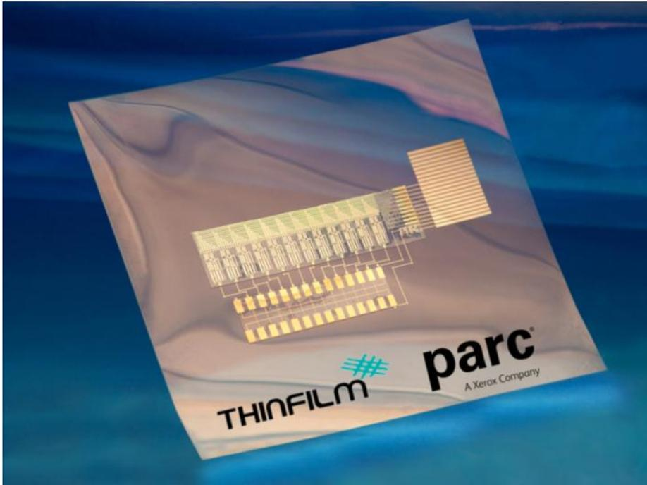
**PRINTED NON-VOLATILE RE-WRITABLE MEMORY:** The addition of integrated circuits makes the roll-to-roll printed Thinfilm Memory addressable by printed logic.
